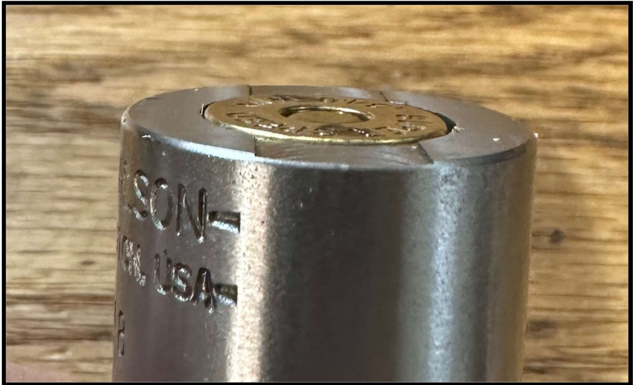
Loaded Round Base is Proud of Max Length Step, will not chamber correctly and allow bolt to lock
