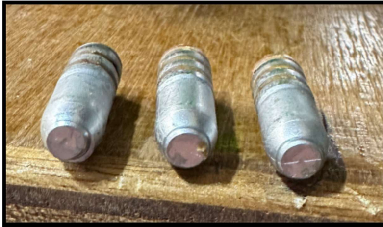
Nose Damage on Accurate 35-250B projectiles using .308" Top Punch
