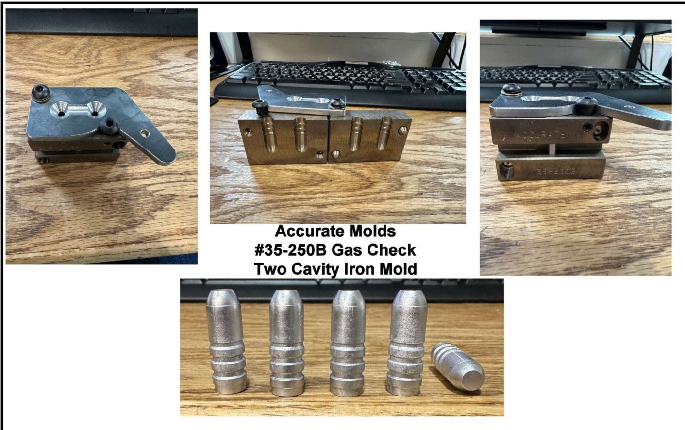
Accurate 35-250B Bullet Mould and bullets cast from Lead
