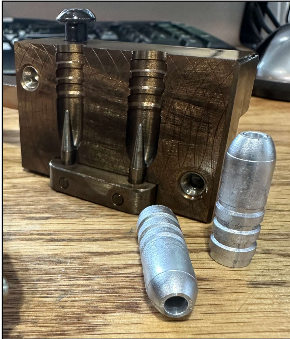
The Accurate 35-250B Mould after Hollow Point Conversion - Weights are ~235grains w/ Gas Check & Lube
