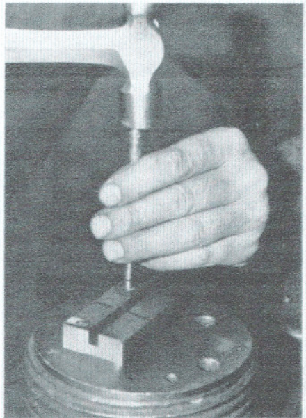
◀ Locked in a special fixture, a pair of blocks are drilled and then moved to this reaming machine for exact sizing of the holes.
