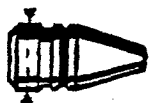
#313 125gr. or 140gr. at BB length. With it's crimp groove, it can also be used as a revolver bullet.
