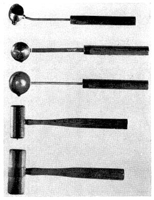
Top: Snout type ladle for use with molds having individual pouring holes. Handle off-set for convenience. Stainless Steel shank keeps the grip cool. Long grip of ample size—does not cramp the hand.
